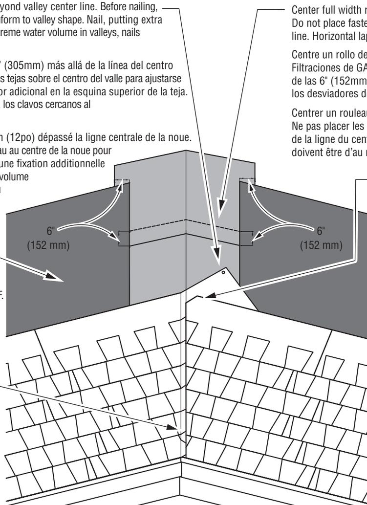
Center full width roll of GAF Leak Barrier. Do not place fasteners within 6" (152mm) of center line. Horizontal laps must be at least 6" (152mm).
